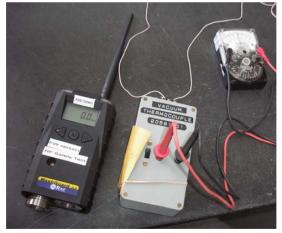
The tests utilized a recently calibrated volt-ohm meter (VOM) meter to measure signal strength; a vacuum thermocouple (VTC) simulated the blasting cap; insulated hookup wire (AWG 22) was used to simulate the lead wires of an electric detonator; and a #2 incandescent light bulb simulated the detonator. During startup of the MeshGuard monitor, the signal-strength meter went full scale, indicating the unit was indeed emitting electromagnetic radiation.
