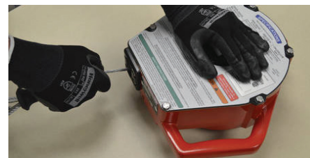
Pull out the entire length of cable until shoulder screws are visible and activate lock.
