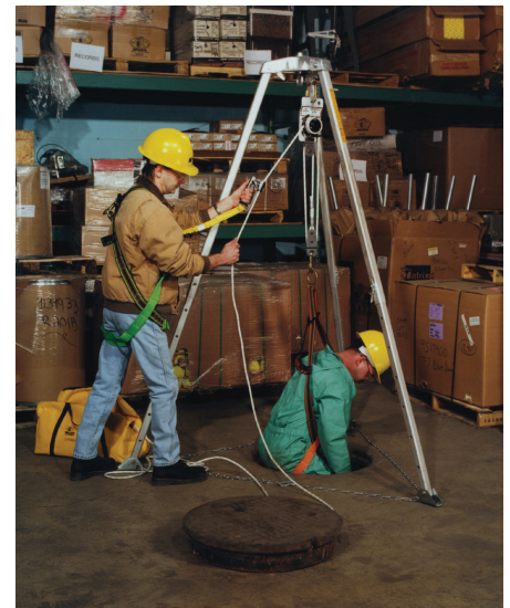
A secondary fall arrest system is recommended
