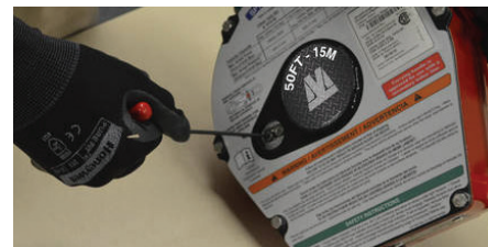
Remove the two shoulder screws on the drum through the side plate cover.
